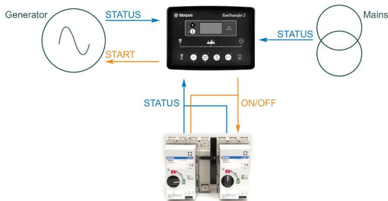
Automatic Changeover System
